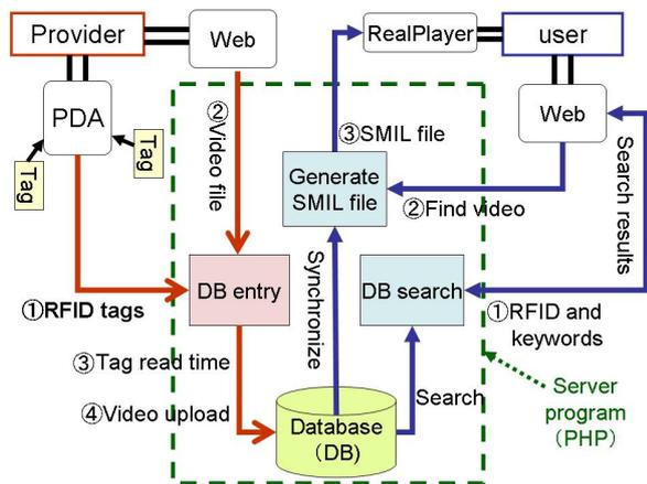
Figure 5: System configuration.
