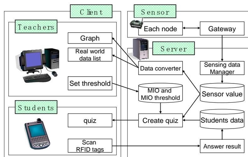
Figure 2. System architecture
