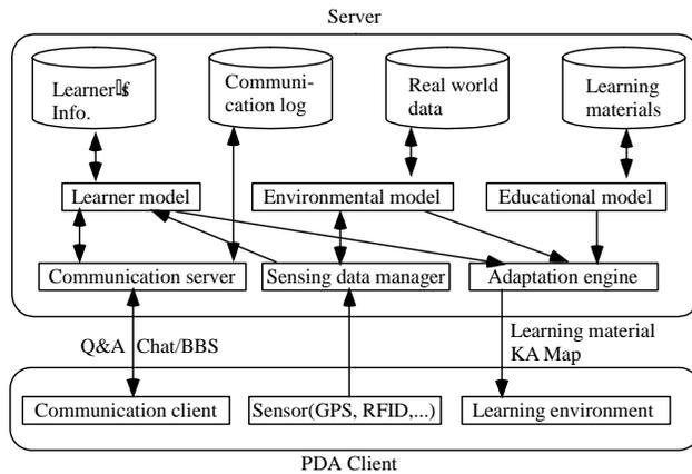
**Figure 6: System configuration of CLUE.**
